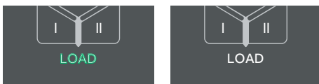
Fig. 3.11 Connected location and I-position: LED is ON, Test location: LED is OFF
